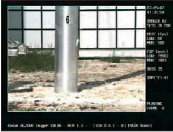
Screen captures of high speed video of Direct Buried FHWA accepted Breakaway Aluminum Pole.
